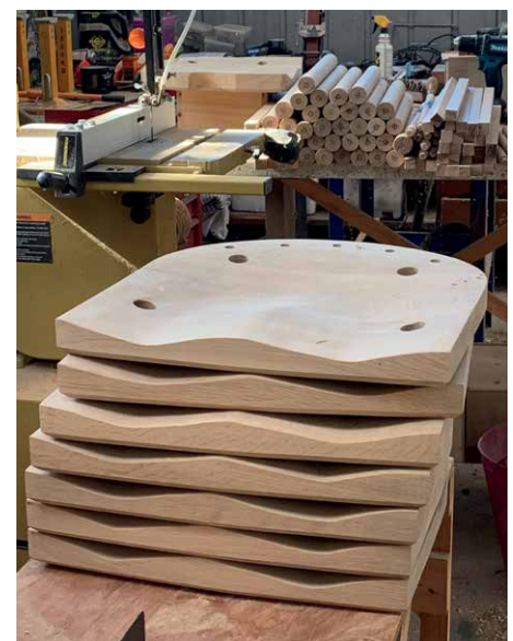
▲ Each seat was fabricated out of three pieces of oak dominoed together and glued with Tite-Bond.
