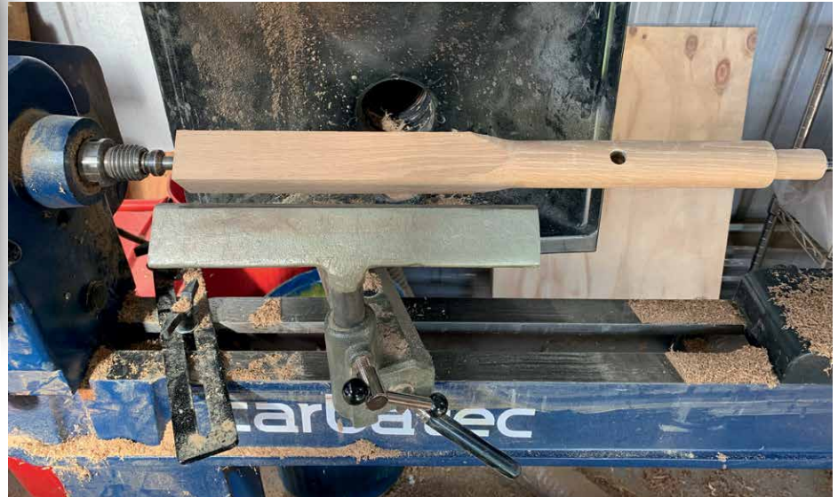
▲ To reduce "chatter" when turning the spindles Paul reduces the speed of the lathe while roughing down to a round. The final cut is done with a large skew chisel.
