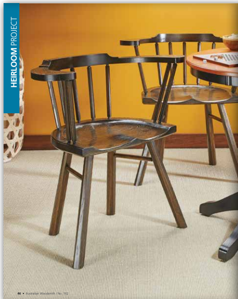
The profile of the back rail mirrors the shape of the seat. The rail curve combined with a centre bridge piece makes the chair comfortable to sit in for extended periods of time. The shaped and contoured seat on the chair looks complicated. But a straight approach and an aggressive cutting disc in an angle grinder make shaping the seat quick and easy.
