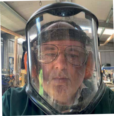
▲ Prescription safety glasses, full visor face shield, earmuffs and ducted dust collection keep Paul safe in his workshop
