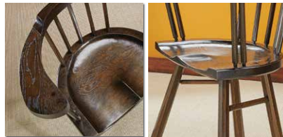
The profile of the back rail mirrors the shape of the seat. The rail curve combined with a centre bridge piece makes the chair comfortable to sit in for extended periods of time. The shaped and contoured seat on the chair looks complicated. But a straight approach and an aggressive cutting disc in an angle grinder make shaping the seat quick and easy.
