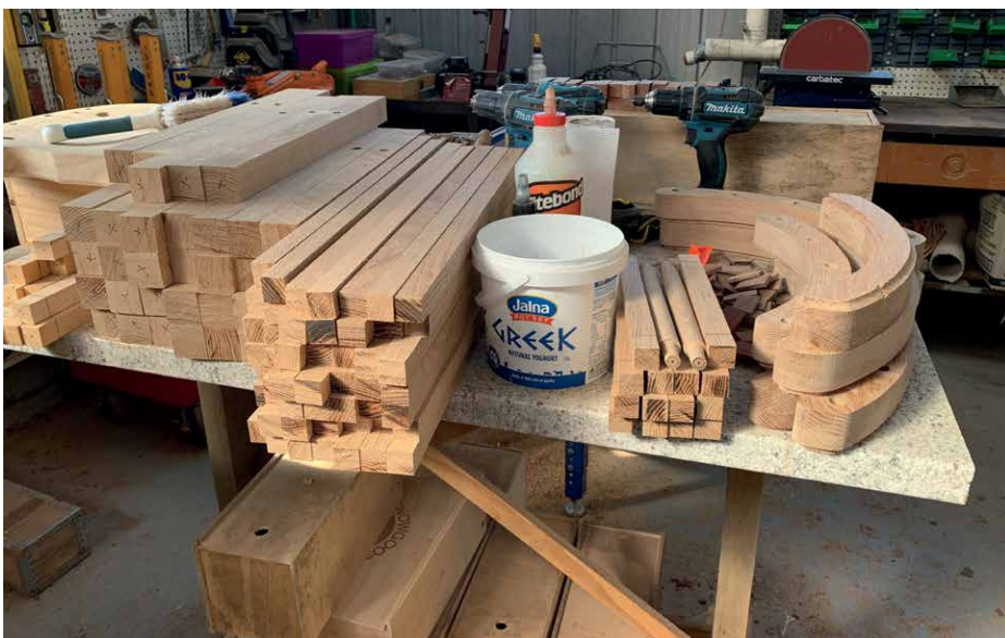
▲ Notice the leg billets to the left have all been predrilled with a drill guide. Paul is systematic with his preparation, planning and execution. The American white oak is kiln dried and stable, making it a good choice for the chairs.
